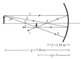
Choose the equation(s) or situation: Use the mirror equation for focal length 2. PLAN and the magnification formula.
