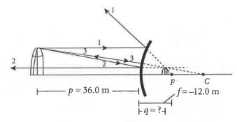
Choose the equation(s) or situation: Use the mirror equation for focal length and the magnification formula.
